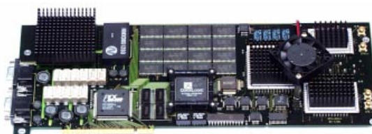
Complete electronics on board - a TCSPC Module of Becker & Hickl
