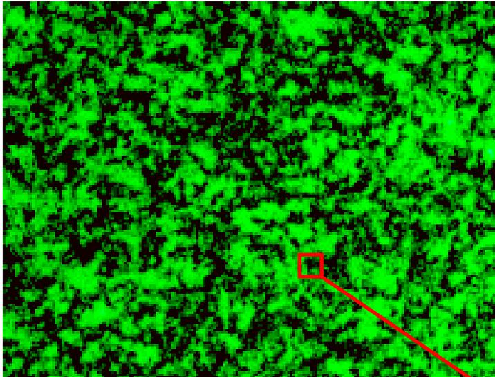
Experimentally, the intensity of one 'speckle' is measured
