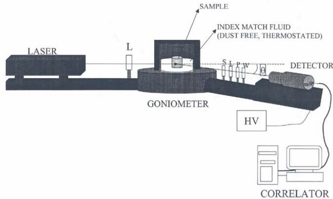
The auto-correlator collects and integrates the intensity at the different delay times,  $\tau$ , all in real time
